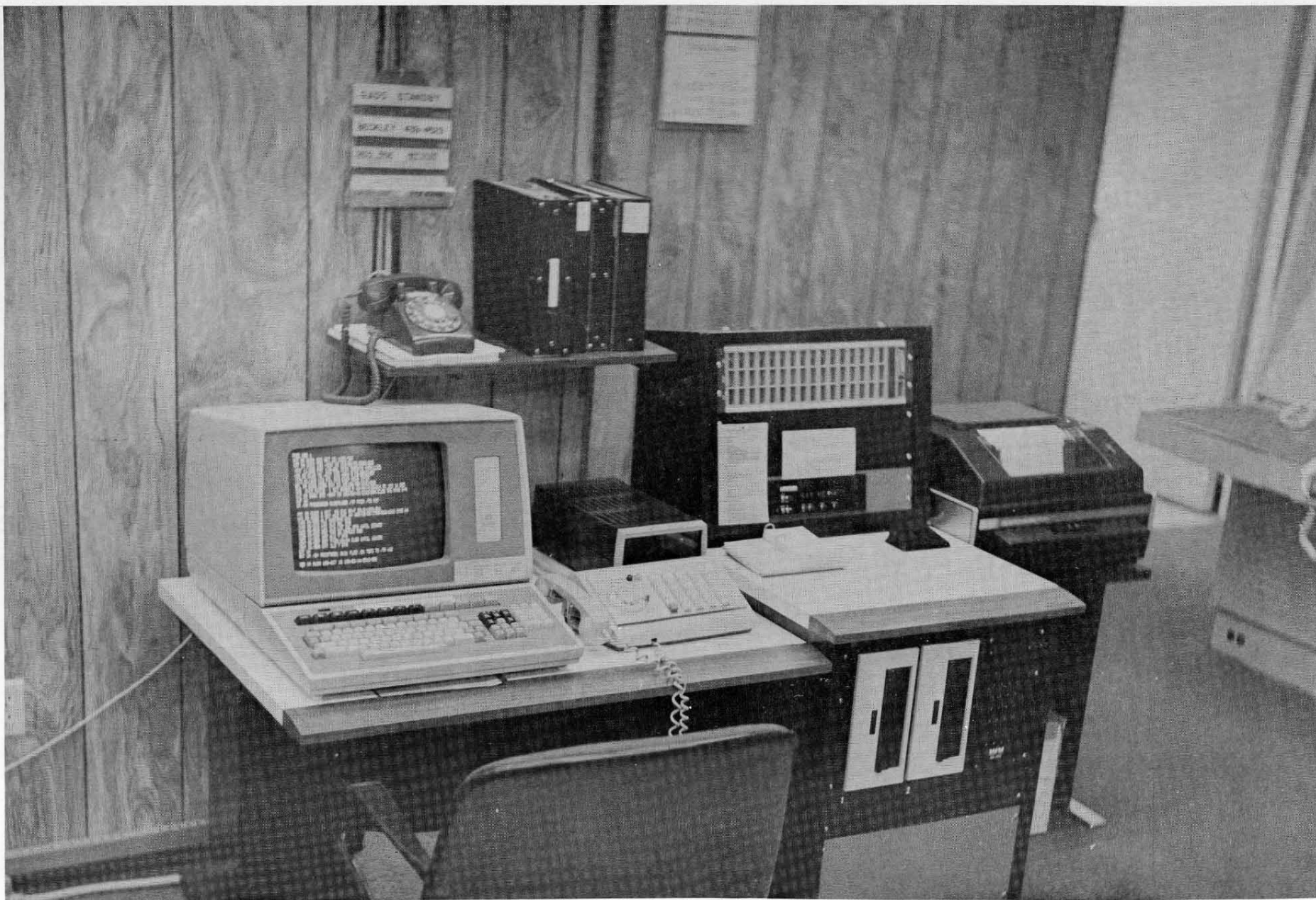
The Western Union "Leased Service A System", with Controller (center-right), Keyboard Display Terminal, and Supervisor Printer (right).
