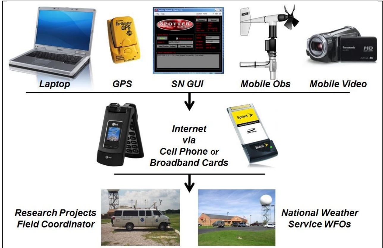
Figure 1. Outline of equipment and accessories utilized by some storm observers providing real-time data to field coordinators and operational meteorologists.
